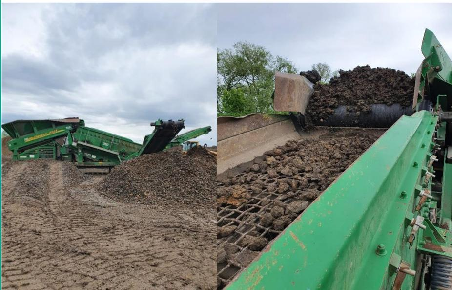
Fig. 1 Mc Closkey sorting machine in action, photo Halík M
