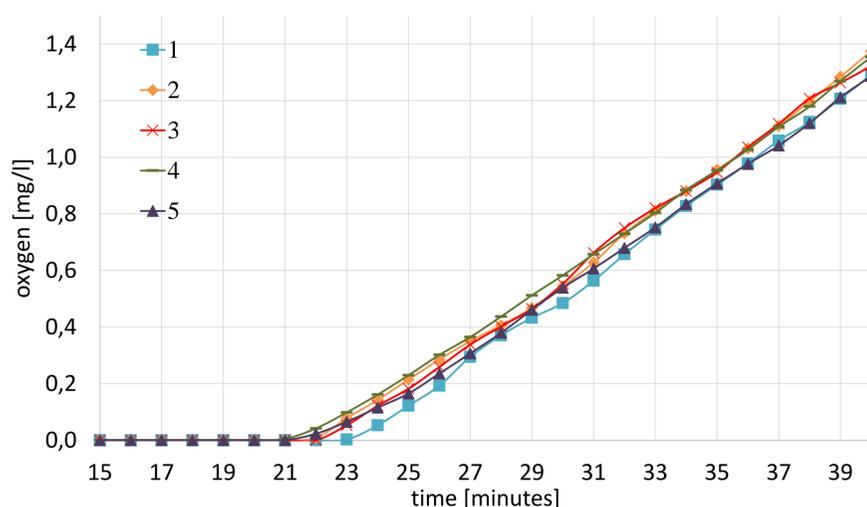
Figure 3. Increase in dissolved oxygen concentration during the first measurement for the five probes.
