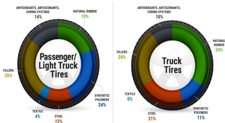
Fig. 1 Composition of tires for passenger and freight transport
